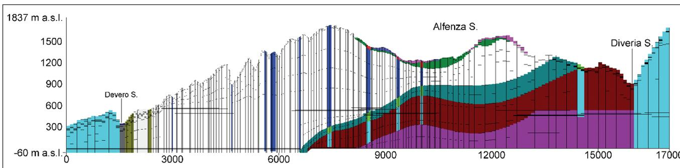
Fig. 5: Section of the model domain along the tunnel trace (N-S direction), column 85: vertical discretization in 20 layers and assigned K zones (according to Table 3); vertical exaggeration of 2:1 is used.
