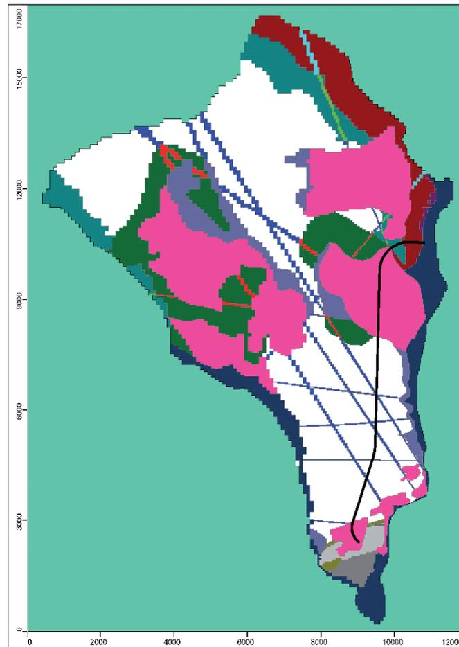
Fig. 4: Flow domain and K zones at layer 1 of the MODFLOW model. Colors corresponding to K zones according to table 3; the inactive cells are represented with the green color; coordinate axis in meters; tunnel trace in black.
