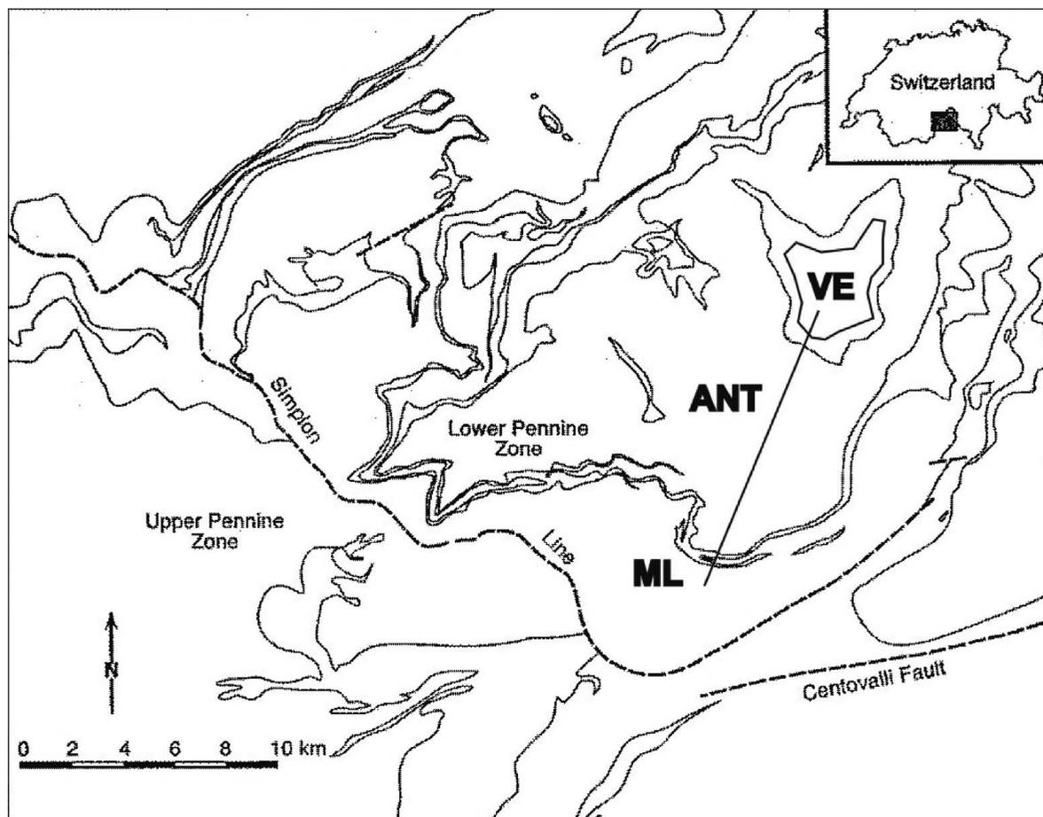
**Fig. 1:** Geological sketch of the area between the Verampio window (VE) and the Simplon Fault (modified from Grasemann & Mancktelow, 1993). ANT: Antigorio gneiss; ML: Monte Leone gneiss. The line represents the trace of the cross section of figures.2 and 3.
